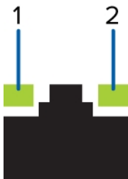
Figure 4: (1) Link LED. (2) Connection Status LED.
